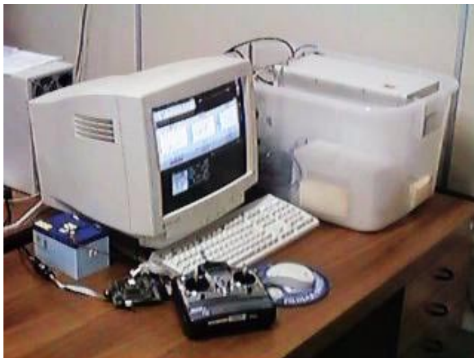
Fig. 7. Ground station with PC, differential GPS and teleoperation unit.
