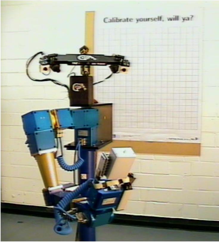
Fig. 1. GripSee's 3 DoF stereo camera head and 7 DoF manipulator.
