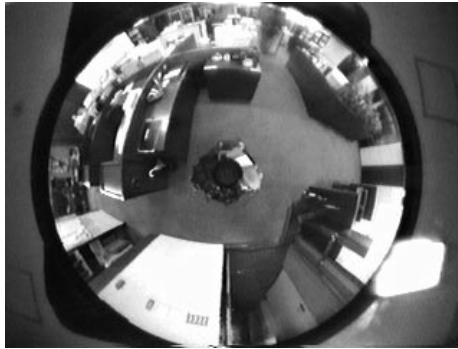
Fig. 2. Typical image from a camera with a hyperbolic mirror
